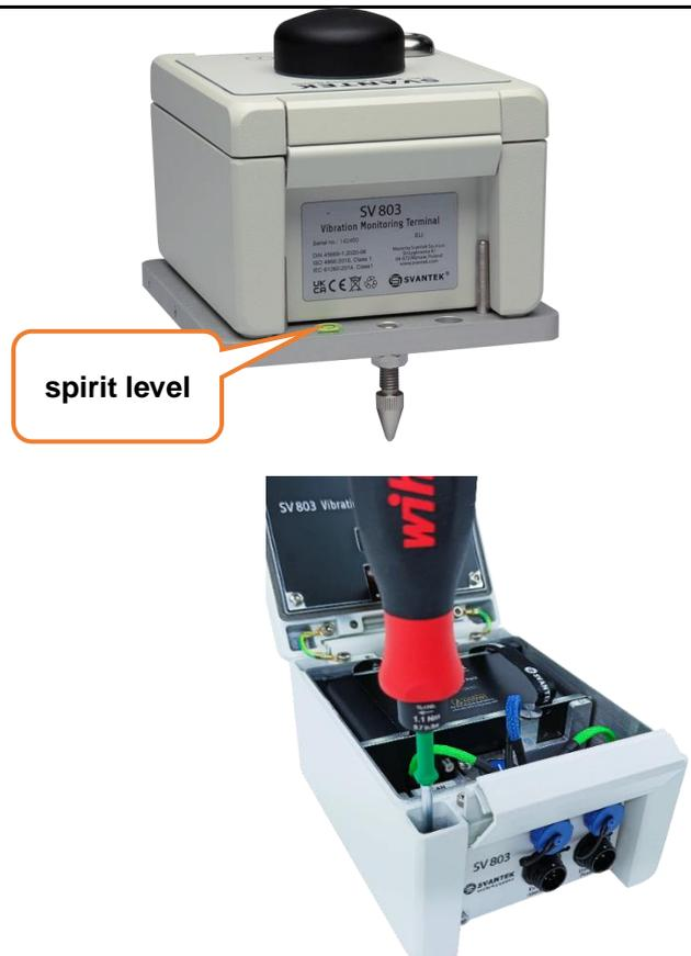
If you wish to mount SV 803 on the wall, you should first attach the mounting base to the wall with the pin trough the central hole in the base.
