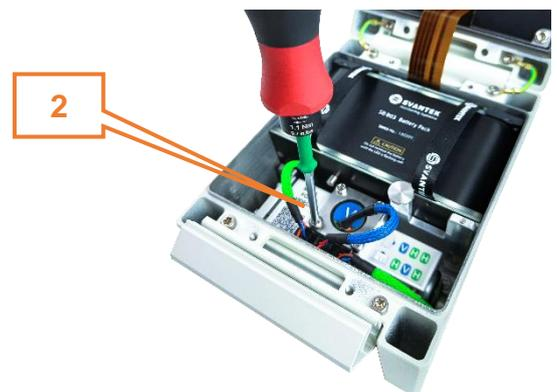
Once the geophone block has been removed, use the torque screwdriver to unscrew the geophone cups and remove the geophone from the box.
