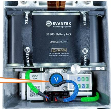
If SV 803 is positioned vertically (usually on the wall), the left geophone must be of the vertical type.
