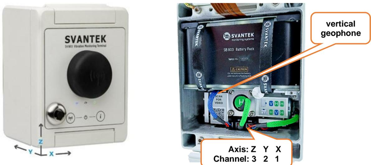
\*) The geophone of the vertical type is equipped with the blue cable!
