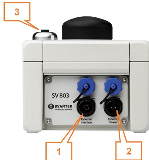
To connect a cable to the WEIPU socket, first align the markings on the plug and socket, then turn the ring near the socket clockwise.
