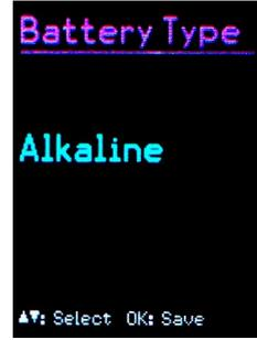
While non-rechargeable batteries have a cell voltage of 1.5 V, NiMH rechargeable batteries deliver only 1.2 V per cell. The VM24 battery indicator can be adjusted to both voltages. To adjust the voltage, open the main menu by pressing F3 and scroll through the menu options by repeatedly pressing the ▼ button until you reach 'Instrument Settings', then press OK.
