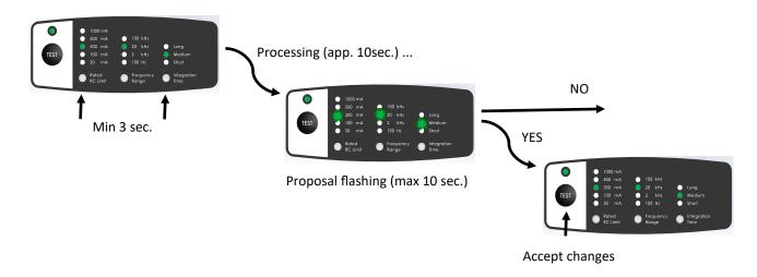
NB: Frequency range of 100Hz is not included in the auto setup feature i.e. if desired the user must select it manually. The RCM will always give priority to settings which make the RCM more sensitive i.e. higher frequency ranges and shorter integration times.
