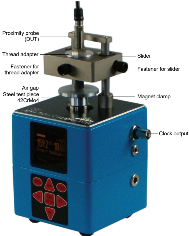
Figure 2: VC21D with clamping device for proximity probes and clock output
