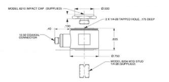
Units on the line drawing are in inches, units in brackets are in millimeters. Refer to 127-1051V for more information.
